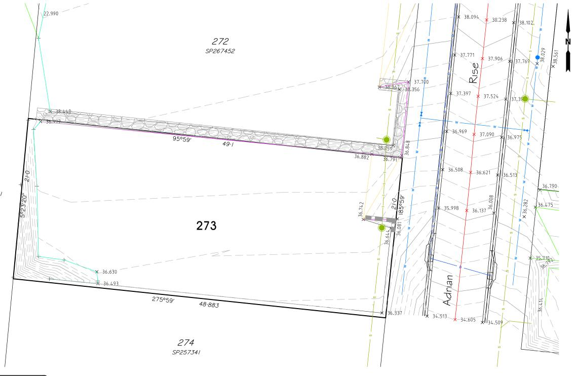
The title boundaries as shown hereon were not marked at the time of survey and have been determined by plan dimensions only and not by field survey. Services shown hereon have been located where possible by field survey. If not able to be located, services have been plotted from relevant authority records and have been noted accordingly on this plan.
